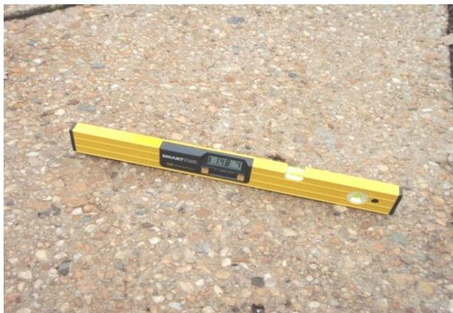
**Level Measuring Curb Cut Slope at 14.8%**
