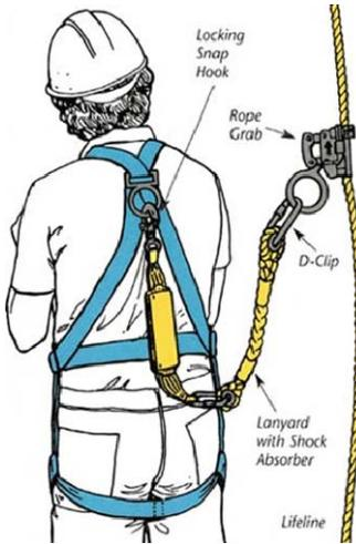
Figure 2: Fall Arrest System
