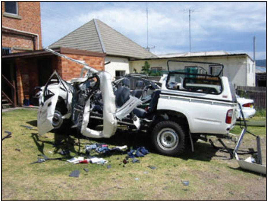
*Figure 3: Result of an improperly stored cylinder.
