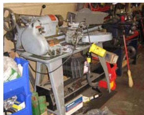
Figure 2: A Plug LO/TO on Metal Working Lathe
