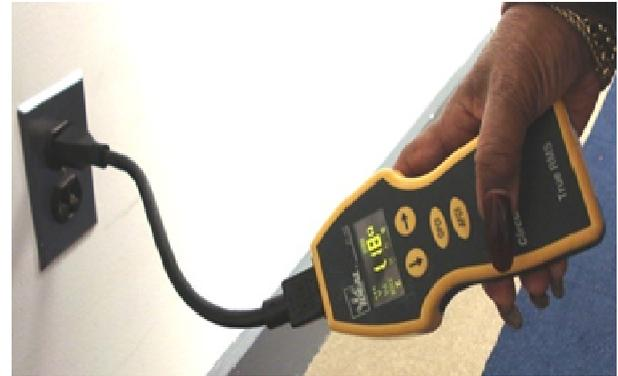
Figure 1: Impedance Tester
